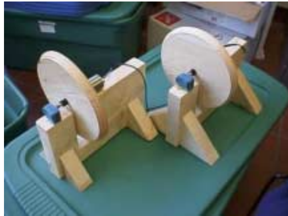
Figure 3.1 Physical system (note that master and slave are identical)
